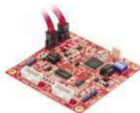
996520PCB&K Integriti UniBus 2 Port RS-232/RS-485 UART PCB & Accessories (Includes 270mm UniBus patch cable)
