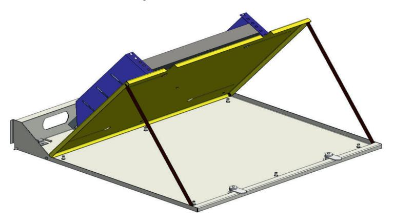
Raise the DVR mounting Plate. Use the 2 supports to keep the plate raised. Use the 4 wing nuts to adjust the mounting brackets to the width of the DVR.
