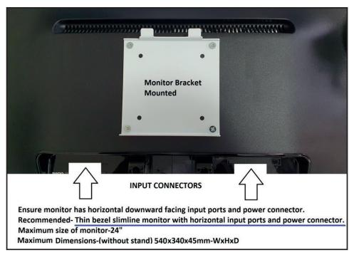
Important Note: if the MONITOR BRACKET shown above fits into a recess on your monitor- you may have to use M4 washers to raise the bracket out of the recess (1 or 2 washers in-between the monitor and the bracket should be fine)
