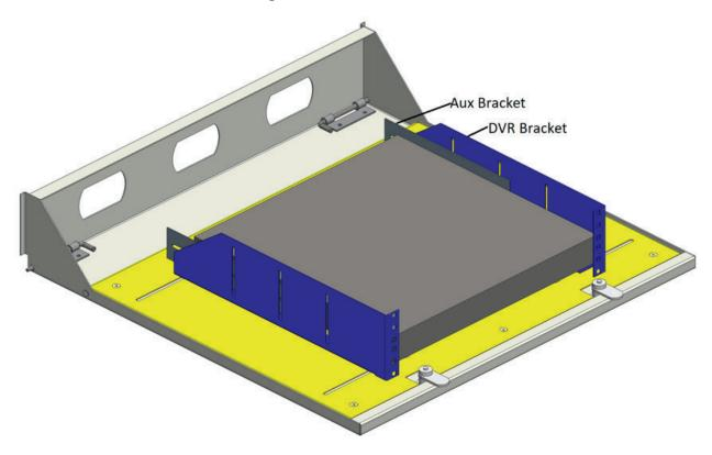
Slightly loosen 4 wing nuts securing the DVR and Aux Bracket together. Move DVR up against the square hole DVR bracket. Then move the Aux bracket up against the rear top corners of the DVR. Secure using the 4 wing nuts. DVR should be secured firmly on the DVR mounting plate.
