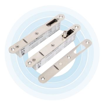
The patented VE1260 is a high torque motor driven drop bolt with up to 35kg pre-load/side load tolerance. It can be installed vertically in the door frame (lock style) or horizontally in the frame header and has a symmetric dead-bolt mechanism to allowing it to be used on 180° degree swing through doors.
