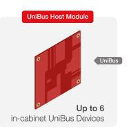
UniBus Devices are designed for installation within the same enclosure as the UniBus host module. A UniBus host can interface a maximum of six UniBus devices in any combination, provided they are all within the intended functionality of the host module
