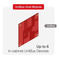
UniBus Devices are designed for installation within the same enclosure as the UniBus host module. A UniBus host can interface a maximum of six UniBus devices in any combination, provided they are all within the intended functionality of the host module
