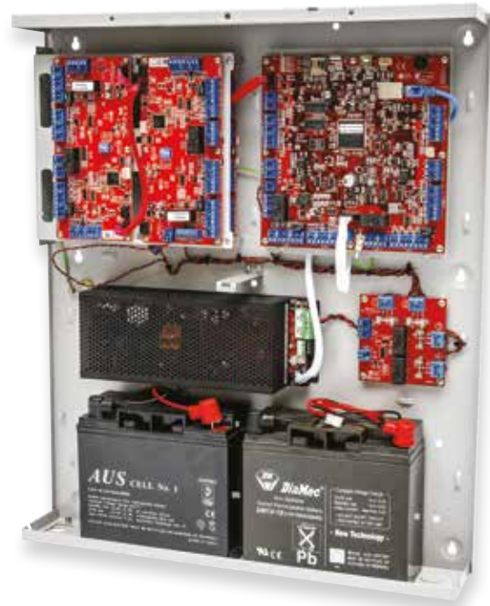
ABOVE: IAC shown in 8 Door / 10 Reader configuration. (IAC with UniBus 2 Door / 2 Reader expansion devices connected). Housed in the WideBody enclosure with hinge plate, 8Amp PSU, Fire Door override relay card and 2x 17Ah batteries
