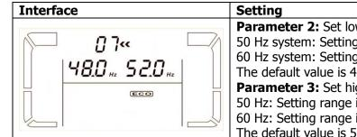
**Parameter 2:** Set low voltage point for ECO mode. 50 Hz system: Setting range is from 46.0Hz to 48.0Hz. 60 Hz system: Setting range is from 56.0Hz to 58.0Hz.
