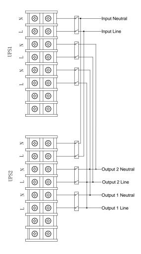
Wiring diagram of parallel system
