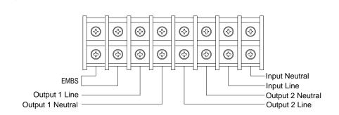
**Terminal Block wiring diagram**
