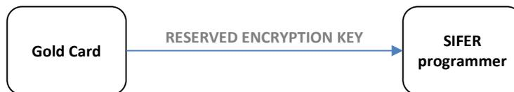
2. Create configuration cards out of SIFER-U user programmable cards to configure the SIFER readers on site with the reserved encryption key
