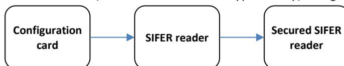
4. Secure the user programmable cards by programming them with the custom site code and the reserved encryption key using the SIFER programmer
