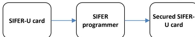
Once the SIFER readers have been configured with the custom encryption key, the SIFER readers will not be able to read SIFER-P pre-programmed cards, only secured SIFER-U cards that have had additional secured data added using the same custom encryption key.
