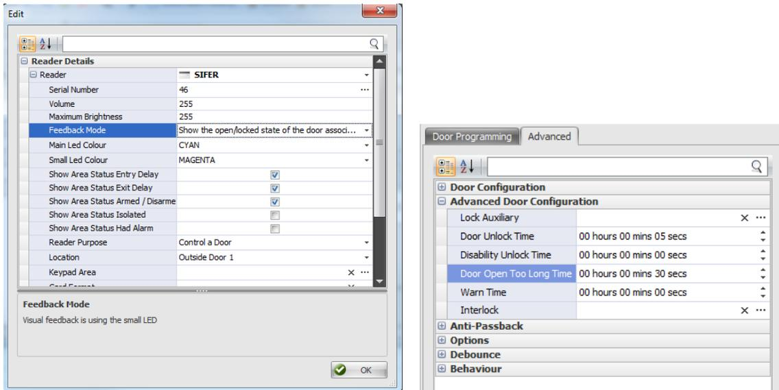
If successfully configured, the SIFER reader associated with the door should provide a continuous pulsating tone when the DOTL system input is in alarm. When the DOTL system input has been restored (i.e. door is closed and reed switch is sealed), the buzzing will immediately stop.
