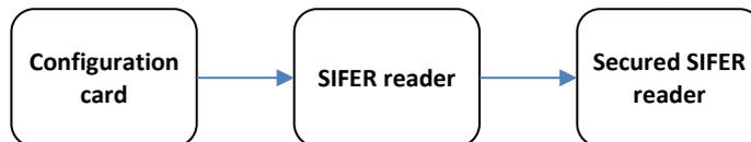
3. Secure the user programmable cards by programming them with the custom site code and custom encryption key using the SIFER programmer
