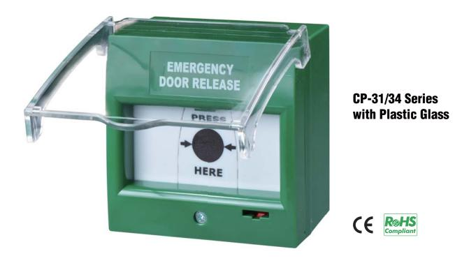
GEM CP-31/34 series call point is a conventional call point that offers double pole, triple pole, or quadruple pole changeover contacts with normally open and closed connections. It is supplied with a breakable plastic glass element that produces no glass fragments to ensure safe and reliable operation. Available in various colors for your choice.
