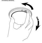
(7) When sensor unit is locked, tighten the tapping screw.
