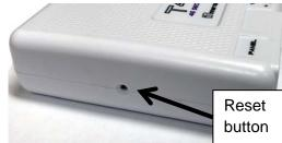
Reset can also be performed by removing power from the unit, waiting 10 seconds and then re- applying the power and battery connections.
