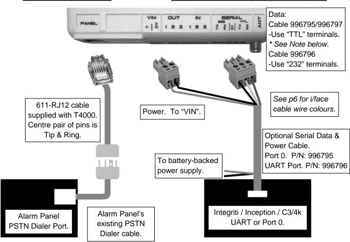
\* **Note:** The early version of the Port0 Cable has a small interface circuit insulated with black heat-shrink sleeve, incorporated into the cable. This version of the cable must be connected to the "232" terminals.
