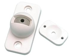
Surface-mount the plastic, low-profile mount to the wall. It is suitable for use with many detector types. The vertical swivel range is  $\pm 10^{\circ}$  to  $-20^{\circ}$ , while the horizontal swivel range is  $\pm 25^{\circ}$ .
