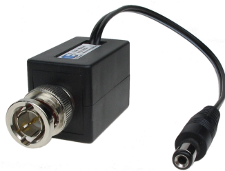
BNC Male to RJ45 Jack with 2.1mm Power Plug Part Number: E10180SP
