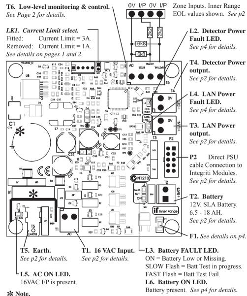
This 3A Smart PS & the legacy 2A Smart PS (no longer available) appear very similar but can be identified as follows: (The current Integriti 2A Standard Power Supply does not support the Smart PS features such as high-level status monitoring)
