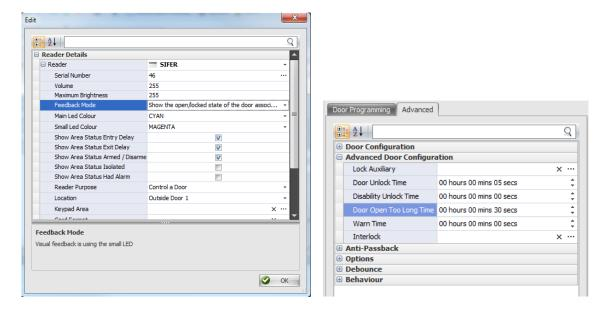
If successfully configured, the SIFER reader associated with the door should provide a continuous pulsating tone when the DOTL system input is in alarm. When the DOTL system input has been restored (i.e. door is closed and reed switch is sealed), the buzzing will immediately stop.
