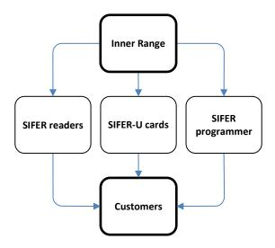
SIFER-U cards are programmed by Inner Range with the Inner Range SIFER Global Key, a default site code of 1001 and a unique card number. As opposed to SIFER-P cards, SIFER-U cards are 'unlocked' and allow credential customisation.
